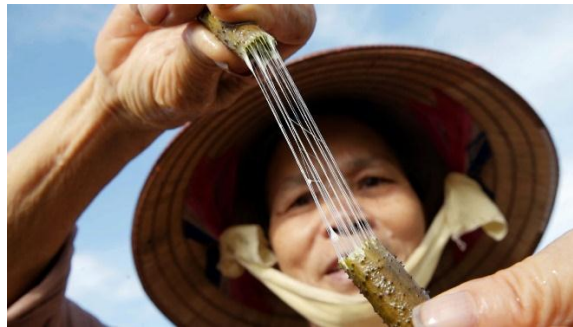
Fig 3. Lotus fiber extracting process
